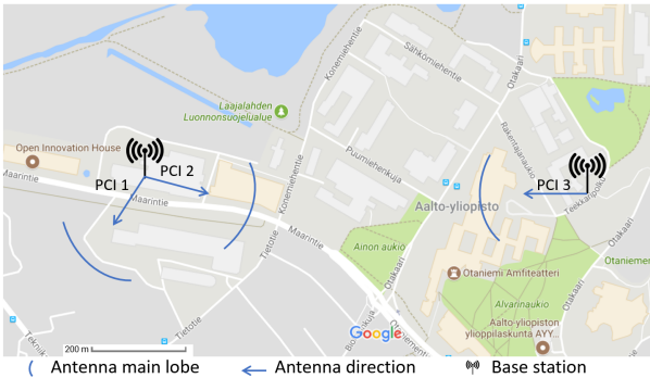
Fig. 1: Map showing the base stations position and the PCIs (sectors) in the reference dataset.
