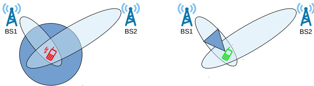
(a) Semi-directional: interference at UE. (b) Fully directional: no interference at UE.
