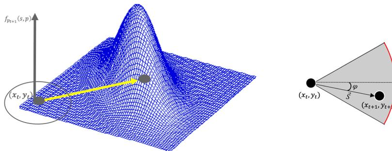
Figure 4: Polar coordinates and predicted position probability distribution.
