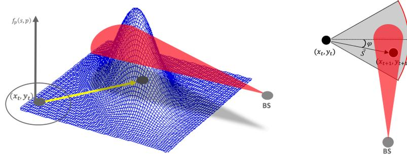
Figure 6: Covered area by the beam  $\mathbf{B}(\theta, \hat{\mu})$  and the probability density function of the predicted position.
