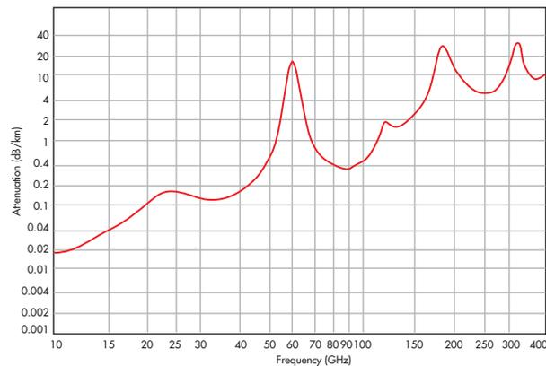
Figure 1: Free-space attenuation on sea-level of radio waves between 10 and 400 GHz. Note that both axes are logarithmic. Figure from [1].
